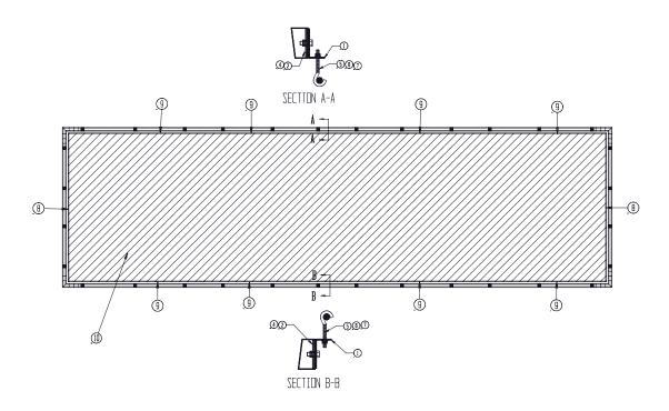
TOP AND BOTTOM GRIPPER BARS REQUIRE THREE PULL POINTS PER BAR SIDE GRIPPER BARS REQUIRE 4 PULL POINTS PER BAR
