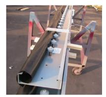
*C. Side Frames* - Signs over 10'6" tall have the Side Frames shipped labeled "Motor End" and "Far End." Signs 10'6" and shorter have the Side Frames shipped attached to the Top Frames. Lower Side
