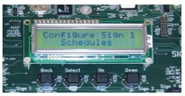
When a sign is in **Run Mode** and the inverter and encoder are properly connected, the green **Run** LED for that sign should be lighted. When a sign is in **Maintenance Mode**, both the green **Run** LED and the red **Maintenance** LED for that sign should be lit. A sign can *only* be configured when in **Maintenance Mode**.
