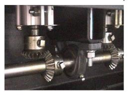
Drive Shaft Coupler. Remove all of the Gears and other Pillow Block Bearing between the location of the Drive Shaft Coupler
