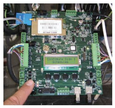
is designed to help ensure the safety of sign maintenance personnel. If a sign is left in **Maintenance Mode** after maintenance is completed, a return trip to the sign will be required to place the sign back into **Run Mode**.
